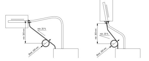
Lead the condensate hose down to the humidifier with a **minimum slope of 20** %, in the form of a **siphon (min. hose bend diameter Ø200 mm )**. Then, lead the hose into the unit through the break-through on the top side of the unit and insert it about 2 cm into the specified opening of the water cup.
