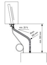
Initially, lead the steam hose with an **upslope of at least 20% over a minimum height of 300 mm** above the top edge of the unit, then lead the hose with a **minimum upslope of 20%** and/or a **minimum downslope of 5%** to the steam distribution pipe.
