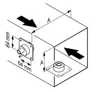
The **steam nozzle W21** can be mounted in the ventilation duct horizontally or vertically. Keep a **minimum distance clearance (A) of 200 mm** between nozzle opening and the opposite duct wall.
