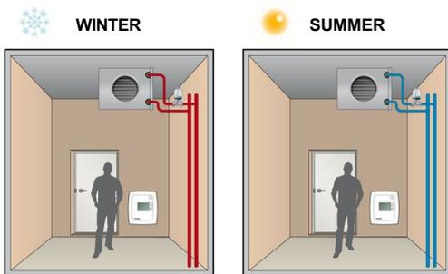
In 4-pipe installations, there are two separate pipe systems for heating and cooling with separate valves. The controller uses two outputs for control of heating and cooling in sequence with two thermal actuators.
