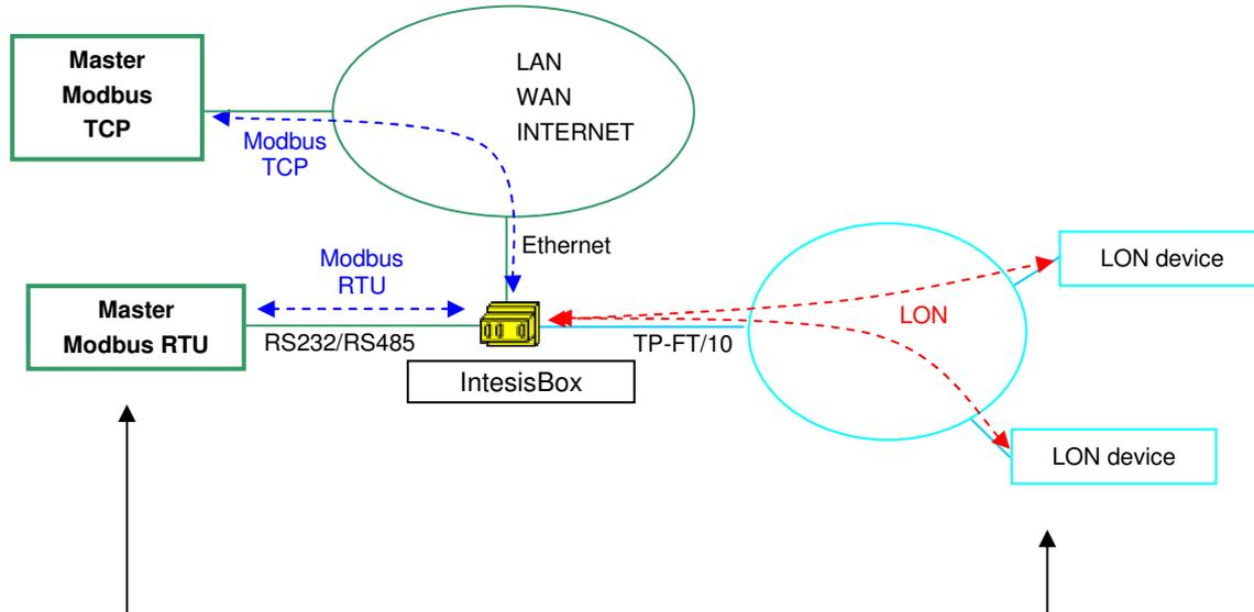
**Control system with Modbus master interface:**
