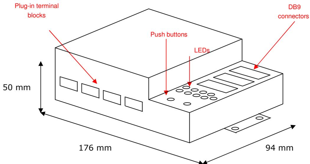
Recommended available space for its installation into a cabinet (wall or DIN rail mounting), with space enough for external connections:
