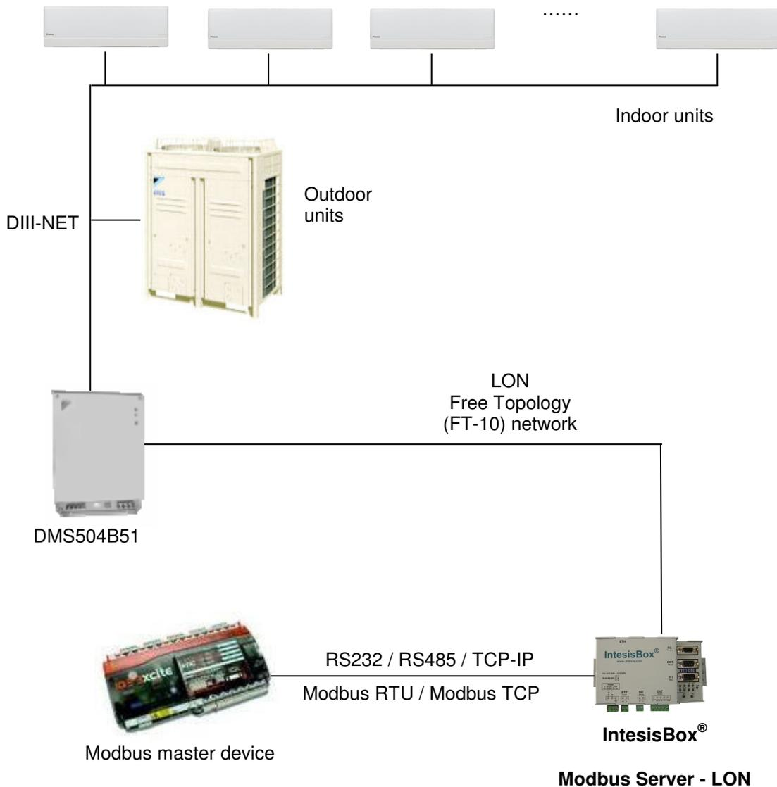
In the technical documentation of IntesisBox supplied with the device, extended details on how to configure IntesisBox for this application is provided.
