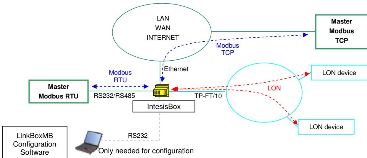
IntesisBox is a Modbus device allowing read/write network variables (SNVTs) of LON devices connected to a LON network, and offering these values through its Modbus interface. **SNVT values in LON can be read/write from Modbus.** Each LON basic data type of network variables in LON devices can be mapped into an individual Modbus register.
