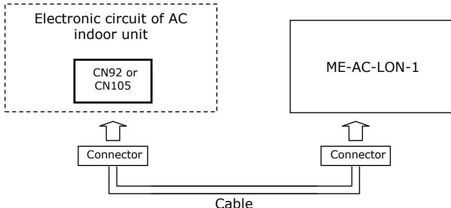
Do not modify the length of the cable supplied with the interface, it may affect to the correct operation of the interface.
