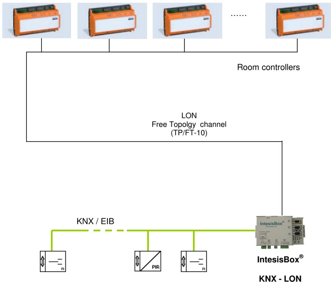
LON network variable interface for each particular LON room controller should be mapped into IntesisBox configuration. *LinkBoxEIB* software eases this task by providing a list of standard network variable types (SNVTs), with their respective fields, which can be assigned to each point.
