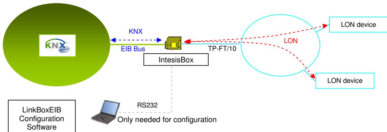
IntesisBox is a KNX device allowing to read/write network variables (SNVTs) of LON devices connected to a LON network, and offering these values through its KNX/EIB interface. **SNVT values in LON can be read/write from KNX.** *Each LON basic data type of a network variable in LON devices can be mapped into an individual KNX group address.*
