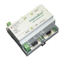
Gateway for monitor and control Siemens FC330A fire detection systems from Modbus master or client devices (SCADA, BMS, PLC, HMI, TouchPanels...)
