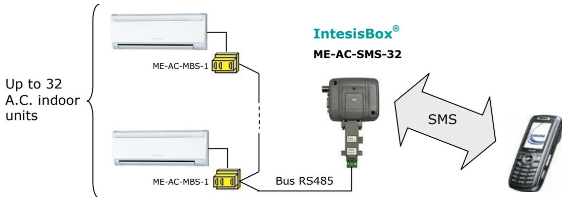
**ME-AC-SMS-32** has been designed to monitor and control Mitsubishi Electric A.C. units using simple SMS messages from any mobile phone or PDA. Compatible with all models of *Domestic & Mr.Slim* lines. Requires the installation of one interface **ME-AC-MBS-1** each A.C. indoor unit to be controlled.
